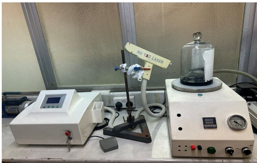
Fig. 3: (A) The PLD setup
