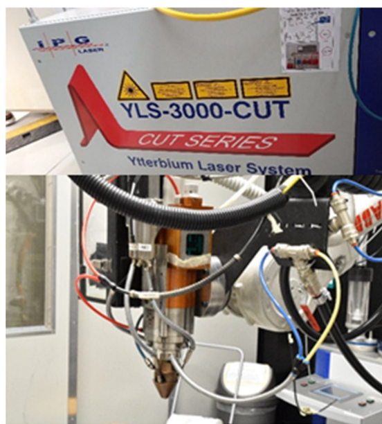
Fig. 4: Ytterbium fiber laser and LDED printhead.
