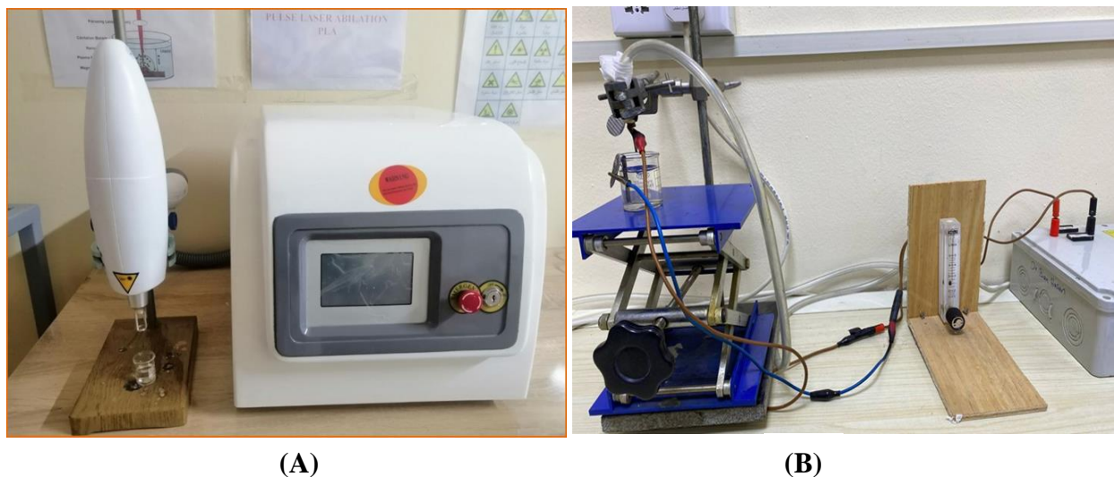
Fig.1. The prepared Ag@Au NPs by a hybrid system (A) Nd:YAG laser (B) plasma jet.
