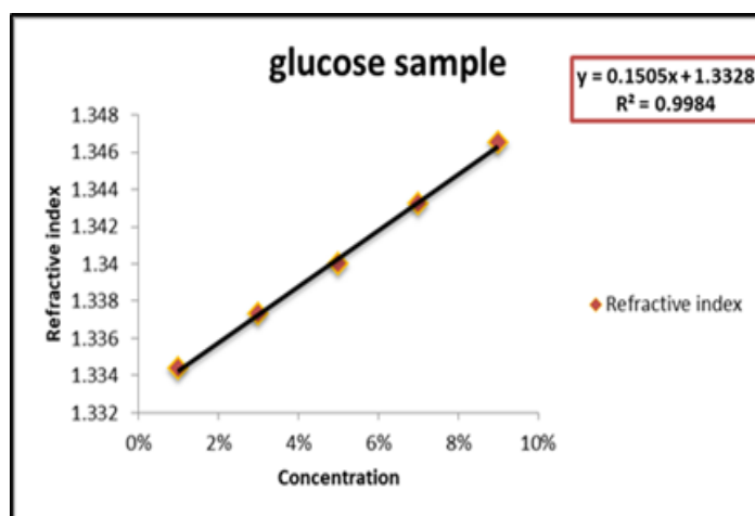
Fig. 4: The concentration of a glucose solution affects the solution's refractive index.
