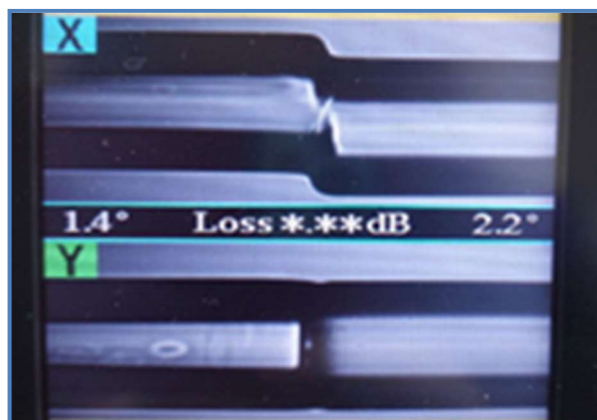
Fig.5: CF-CF offset splicing.
