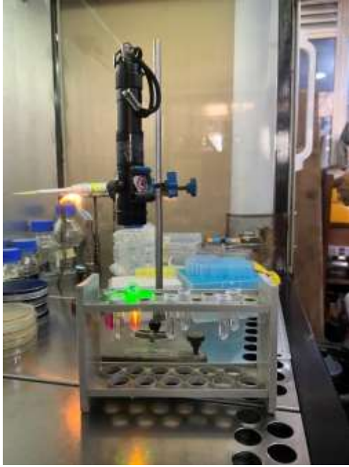
Figure (2): Irradiation of S. aureus by a diode laser with Rose Bengal
