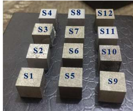
Fig. 1: SLM as-manufactured specimens.
