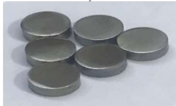
Figure (1): Titanium discs were grinded and polished using silicon carbide papers in sequence of 120, 320, 500, 800, 1200, 2000 and 2400 grit size to obtain a uniform surface)
