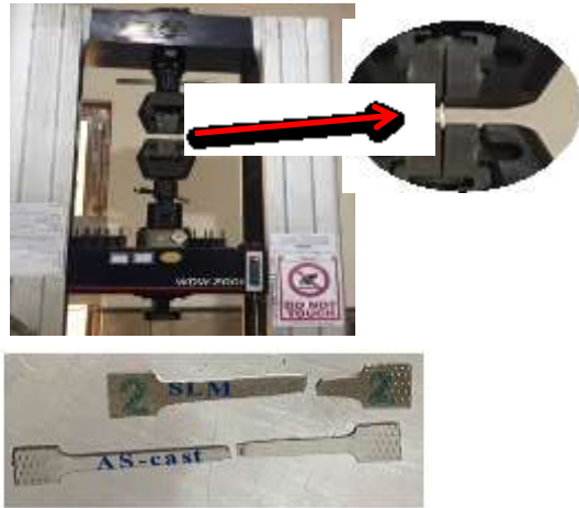
Fig. 15: The tensile testing machine for tensile testing, samples after testing
