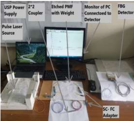
Figure (3): The experimental setup for Sagnac interferometer with loop MZI- PM.
