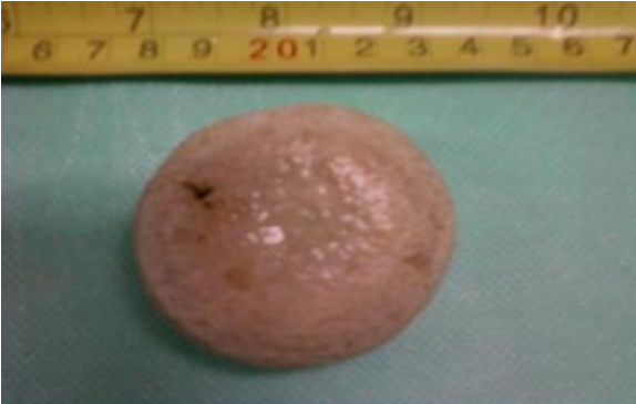
(C) Step 1 : P.E=0.4J, PRR=25Hz, p=20 weight=66.73 gram weight loss=0.13 gram
