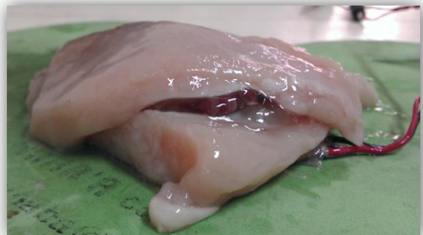
Fig. (5): The phantom (2 pieces of chicken breast issue and fish heart as a tumor)
