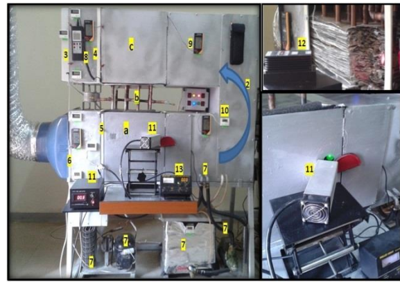
Fig (2): complete test rig of thermosyphon heat pipe heat exchanger. 1. Heat pipe heat exchanger (HPHE)a. Evaporator section b. Adiabatic section, c. Condenser section,2. U Duct,3. Fixed variable speed Fan,4. Rotated plate,5. Air filter,6. Air heater,7. Chilled water coil system(CWC),8.Digital anemometer,9.Terminator, 10.Thermometer, 11. Diode laser with wavelength 532nm, 3W power,12 .Diode laser with wavelength 650nm, 0.13W power, 13.Detector .
