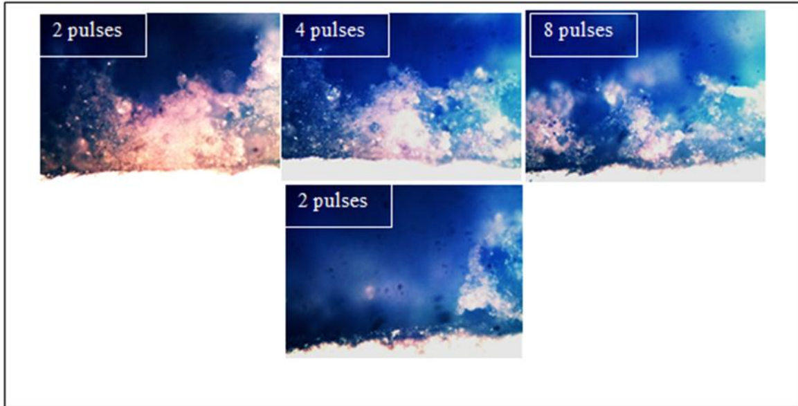
Fig. (2): Microscopic cross section image of iron plate cleaned with different number of Nd:YAG laser pulses and 9.17 \times 10^{10} \text{ W/cm}^2 laser intensity.
