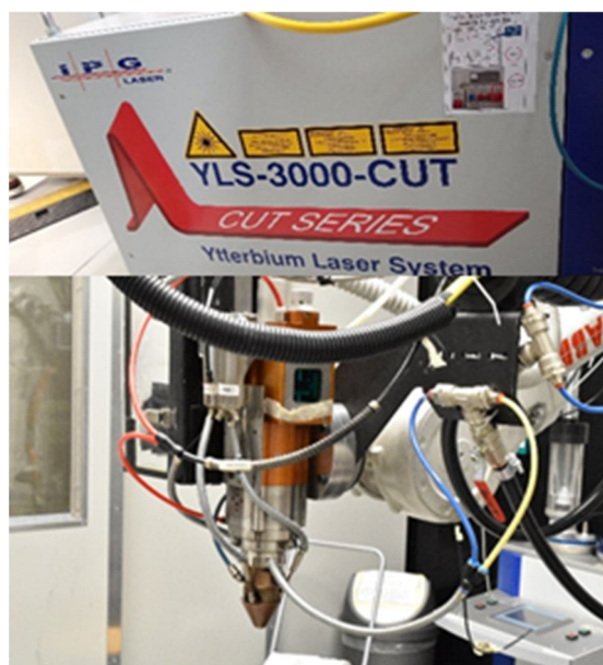
Fig. 4: Ytterbium fiber laser and LDED printhead.
