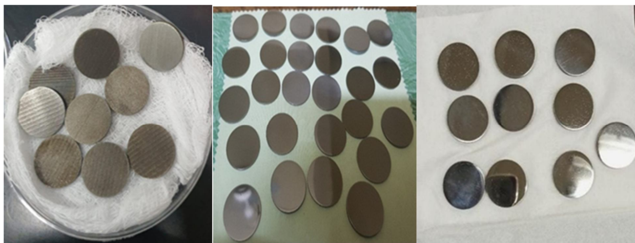
Fig.1: Photograph of mirror-polished Ti6Al4V alloy specimens after sequential grinding and polishing, showing smooth reflective surfaces used for laser surface modification experiments.
