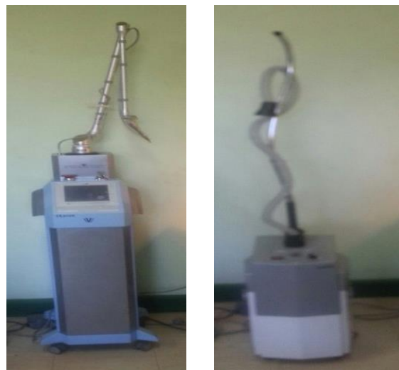
Fig. (1): ( A) The CO 2 laser device (ultra dream pulse V, :DS-40U, Daeshin enterprise), ( B) The smoke evacuator used in this study.
