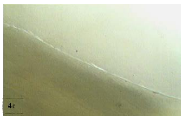
Fig. (4-c): Group 4. Sample at score 3 revealing no dye penetration at the floor of the cavity, magnification X 60. 4c
