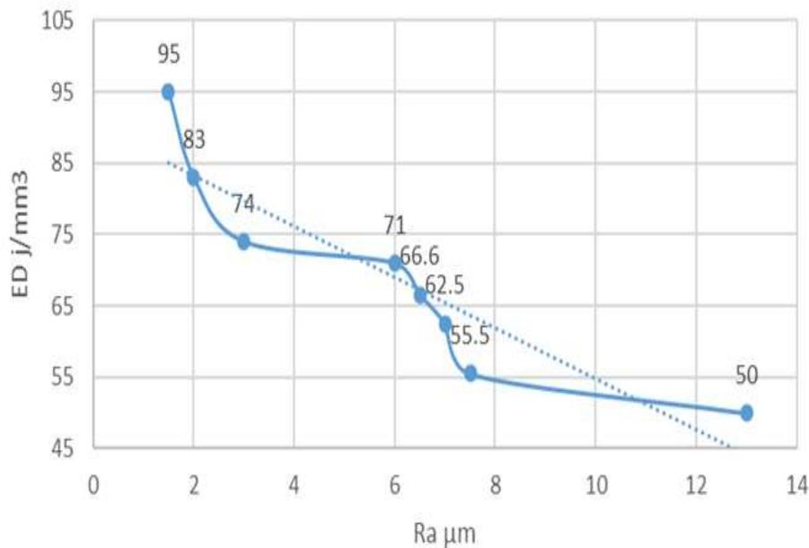
**Fig. 8:** Surface Roughness of Co24.7Cr5Mo5.4W alloys produced with SLM using various energy density after mechanical grinding.
