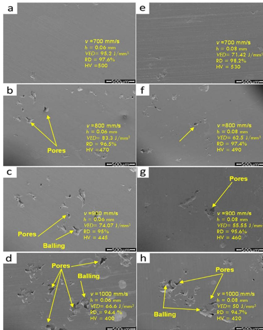
**Fig.3:** SEM images for Co<sub>24.7</sub>Cr<sub>5</sub>Mo<sub>5.4</sub>W alloy samples produced with different sets of process parameters after mechanical grinding.
