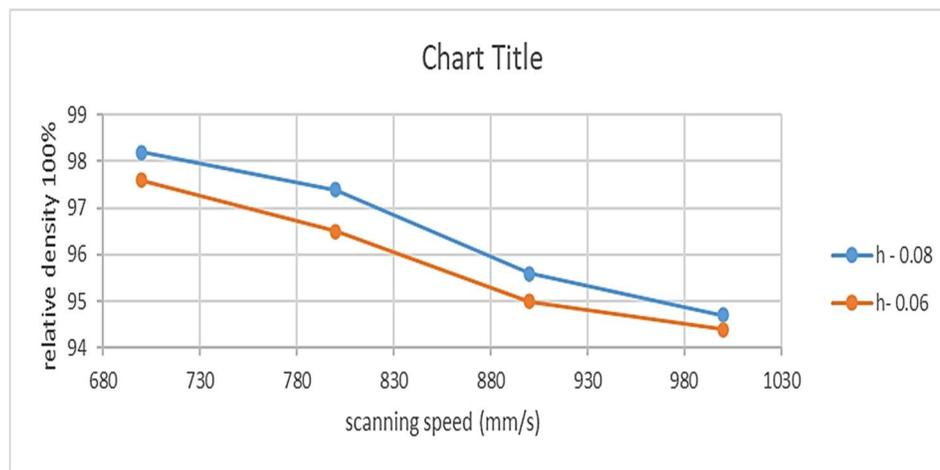
**Fig.2:** shows density curves for SLM-created Co<sub>24.7</sub>Cr<sub>5</sub>Mo<sub>5.4</sub>W alloys at a range of laser scanning speeds.
