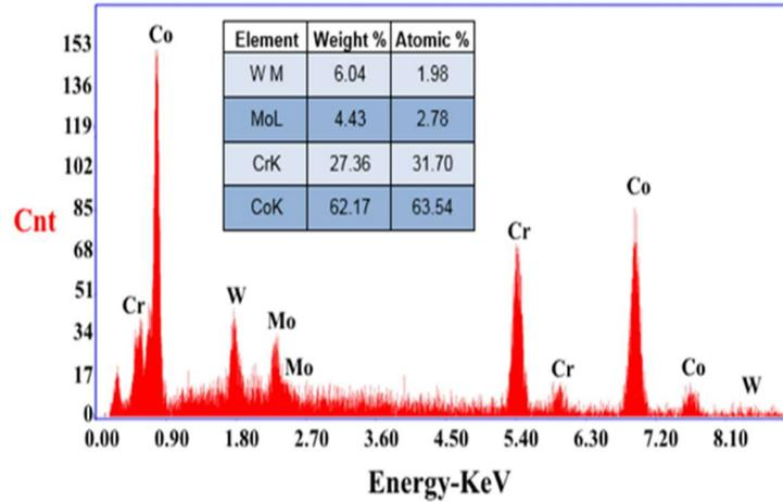
Fig. 5: EDS image spectrogram of Co<sub>24.7</sub>CrWMo.
