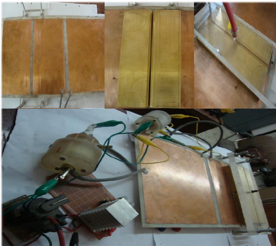
Fig. (7): (b). Two stage Blumlien TEA N2 Laser system.
