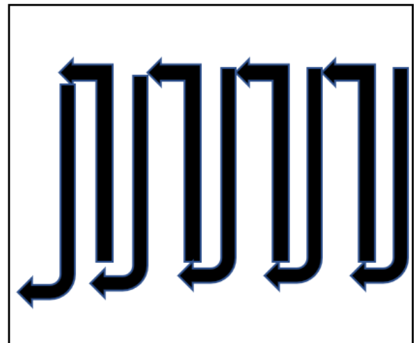
Fig. 3: scanning strategy of fiber laser zig-zag shaped wave..
