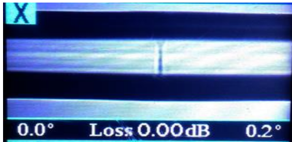
Fig. 2. The splicing region between SMF and CF using automatic splicing mode
