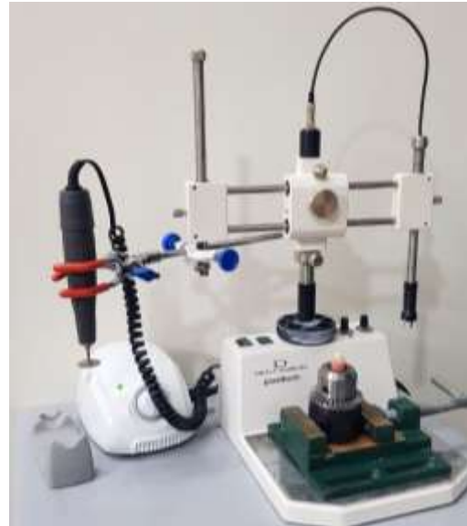
Figure (1) Teeth preparation set-up with the dental surveyor, diamond disc for cutting.
