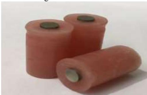
Figure (3): Acrylic molds of titanium discs which embedded to depth of 2 mm and about 1 mm from disc height was remained uncovered to guarantee that Ti disc remain intact throughout cementation.
