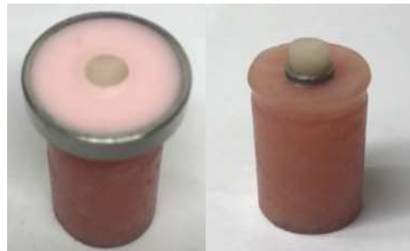
Figure (5): Cementation procedure performed by dispensing an equal volume of resin cement through mixing tip and distributed through the mold opening then photopolymerized by light curing device.
