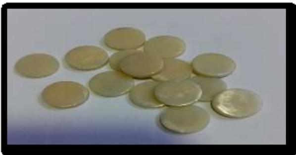
**Figure (1):** Milled zirconia disc specimens.
