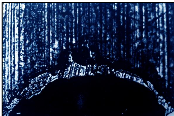
Fig. (4): The resolidified metal on the rims of the laser-drilled hole under atmospheric pressure (X200).
