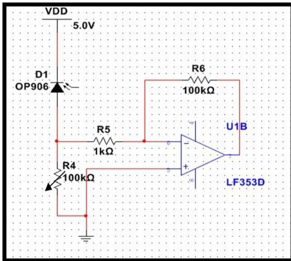
Figure 2 the photodetector simulation by electronic workbench.
