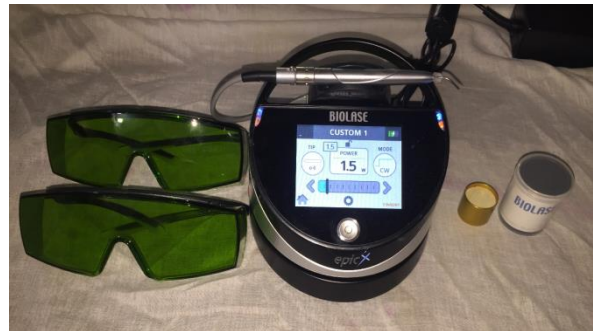
Fig. 3: Laser device with its accessories (eye goggles and initiation kit for laser tips)
