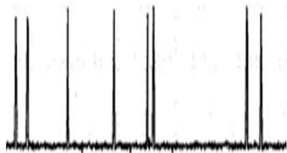
Fig.(3): The random time of arrival of consecutive photons of attenuated laser source [7]
