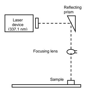
**Fig** (1) Set-up of irradiation of samples by laser.
