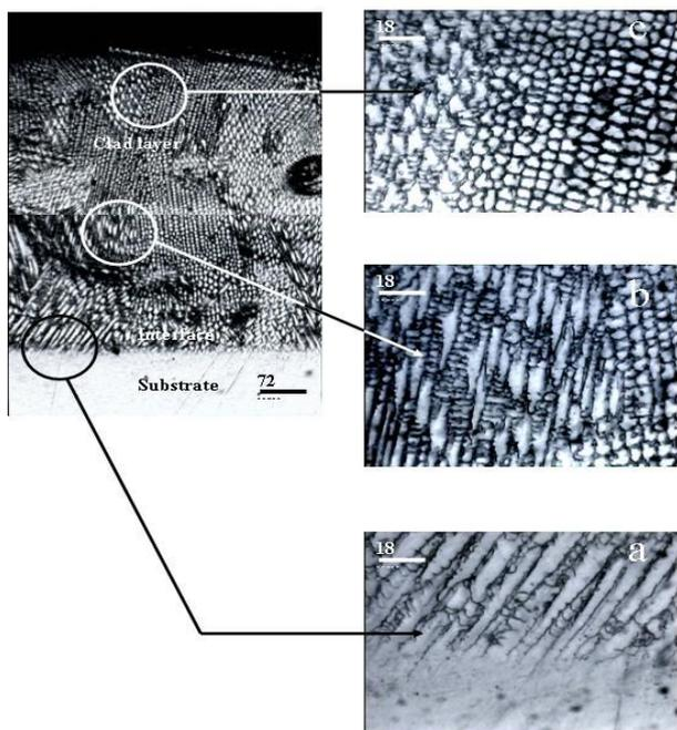
**Fig. 7:** Microstructure of laser clad Inconel 617 substrate with Ni-10%Al premixed clad powder at cladding speed of 13.3 mm/s, (a) clad layer/substrate interface region, (b) central region of clad layer, (c) near external surface of clad layer.
