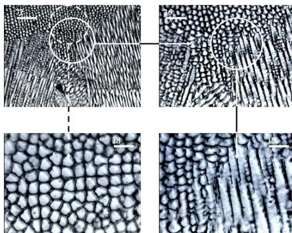
**Fig. 5:** Microstructure of clad layer central region of laser clad Inconel 617 substrate with Ni-10%Al premixed clad powder at cladding speed of 5.3 mm/s.
