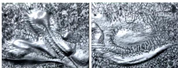
**Fig. 11** Microstructure of some microstructural segregation that developed in some positions of clad layer central region of laser clad Inconel 617 substrate with Ni-30%Al premixed clad powder at cladding speed of 7.3 mm/s.
