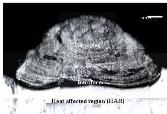
**Fig. 1:** Macrostructure of clad layer of laser clad Inconel 617 with Ni-10%Al premixed clad powder at cladding speed of 5.3 mm/s.
