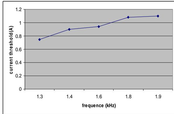
Fig. (4): The effect of increasing pulse frequency on thin disc laser threshold current
