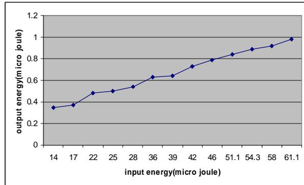
Fig. (5): The relation between input energy and output energy of the thin disc laser at 1.3 kHz pulse frequency.
