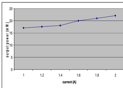
**Fig. (7):** Relation between output power of the diode laser (808 nm) "pumping power" and output power of the thin disc laser (1064 nm)
