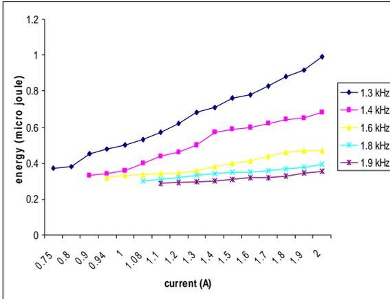
Fig. (2): The relation between input current of the diode laser with output energy of the thin disc laser at different frequencies.
