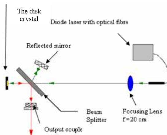
Fig. (1): Thin disc laser setup
